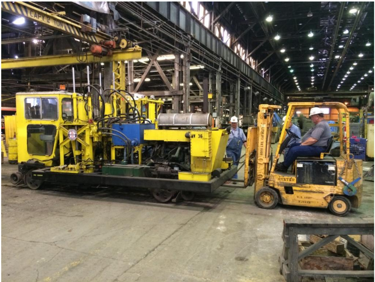
Gene moving the tie-shear out into the center aisle of the Boiler shop
